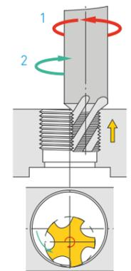
When climb milling, the chip thickness at the end of cut is always 0 ( $h=0$ )
