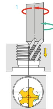
When conventional milling, the chip thickness at the end of cut is always at maximum ( $h=\max$ )
